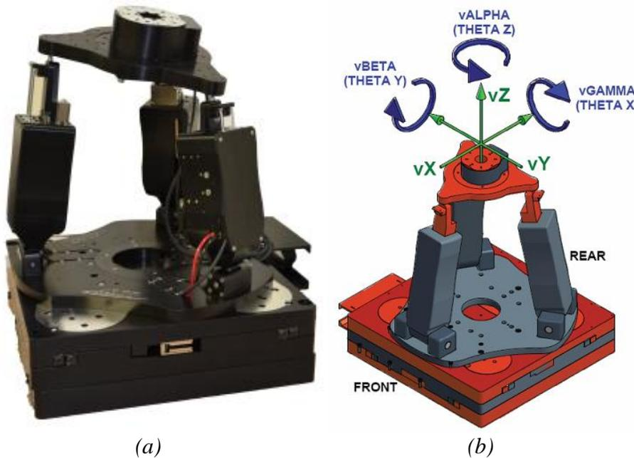
Figure 2. Example of (a) the ALIO Hybrid Hexapod, and (b) the six degrees of freedom of motion capable with the Hybrid Hexapod.
