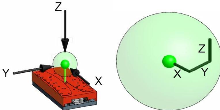
Figure 5. An example of a spherical tolerance zone that represents the X, Y, and Z components of the repeatability distribution in three-dimensional space.
