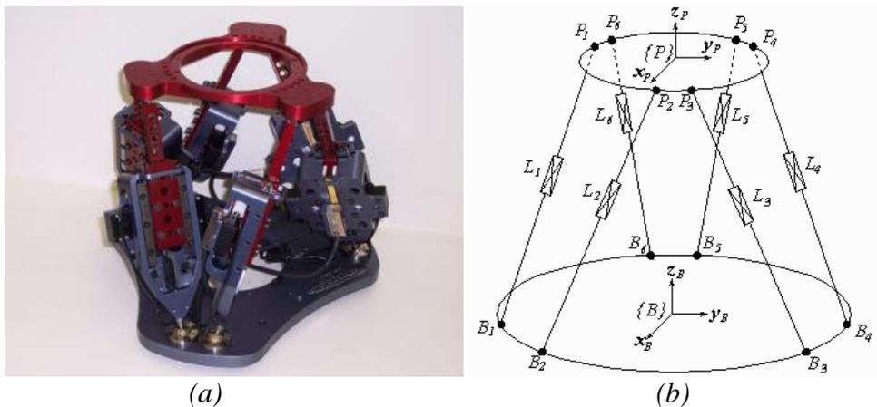
Figure 1. Example of (a) the ALIO HR2 hexapod model, and (b) the six link parallel kinematic layout common to hexapod motion systems.
