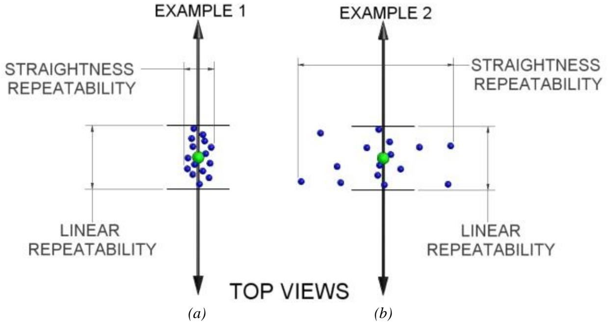
Figure 4. Two examples of repeatability distribution in two dimensions or measurement directions. Clearly the linear repeatability along the axis is equal, but only if the straightness repeatability (perpendicular to the axis of travel) is shown/tested is the difference quantified.
