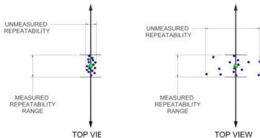
FIGURE 3. Two independent representations of repeatability of a linear axis in a 2D plane.
