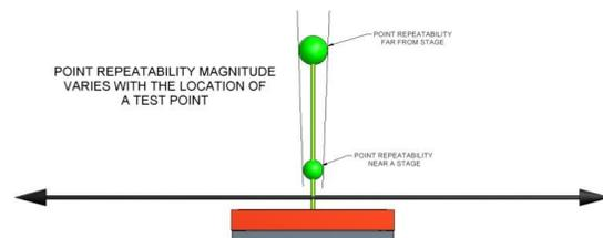
FIGURE 6. A visual representation of the impact pitch repeatability will have on actual point repeatability magnitude recorded.
