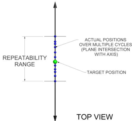
FIGURE 2. Traditional repeatability test method and theory results in a range of points along an axis, which characterizes one-dimensional linear repeatability.
