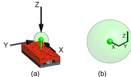
FIGURE 4. A representation of (a) X, Y, and Z repeatability components of a functional point attached to a motion carriage and (b) the spherical tolerance zone that will encapsulate all positions of the test point.
