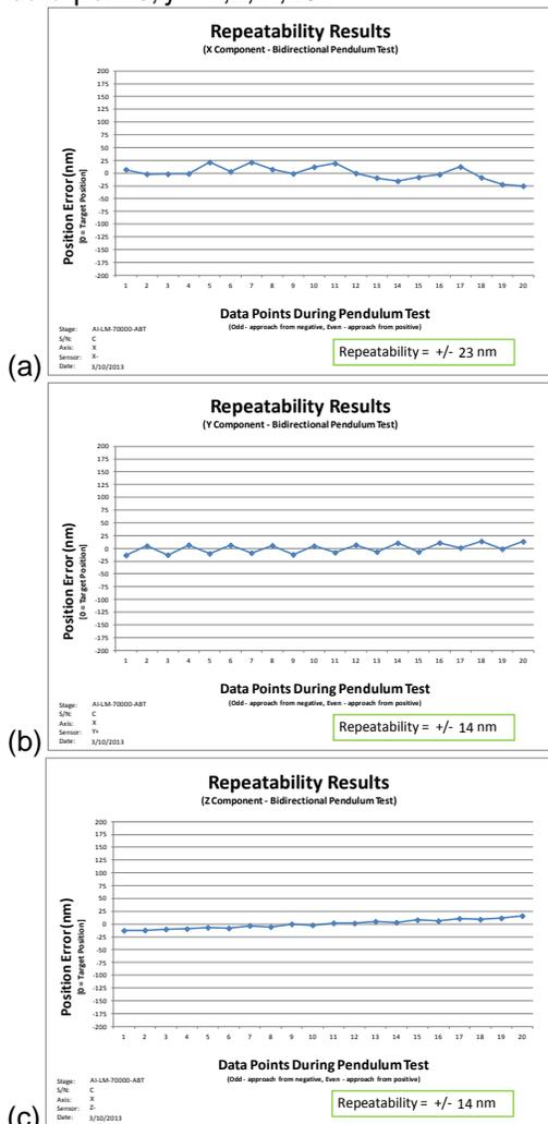
FIGURE 7. The (a) X, (b) Y, and (c) Z components of the raw repeatability for target point,  $i = 5$ .
