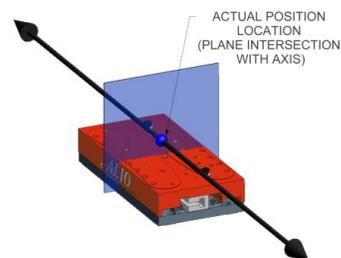
FIGURE 1. The intersection of a plane (fixed to a moving carriage) along an assumed perfect axis is a positional data point used in traditional repeatability testing.
