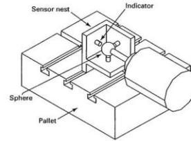
Fig. 7.43 Three-Sensor Nest Setup for Tool Change Repeatability
